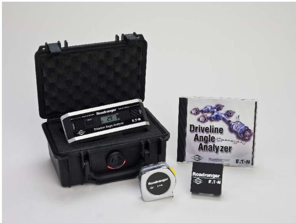
Improper driveline angles can be the source of uncomfortable and destructive torsional vibration. Being able to measure these angles correctly is the first step in diagnosing a problem and ultimately taking corrective action.
