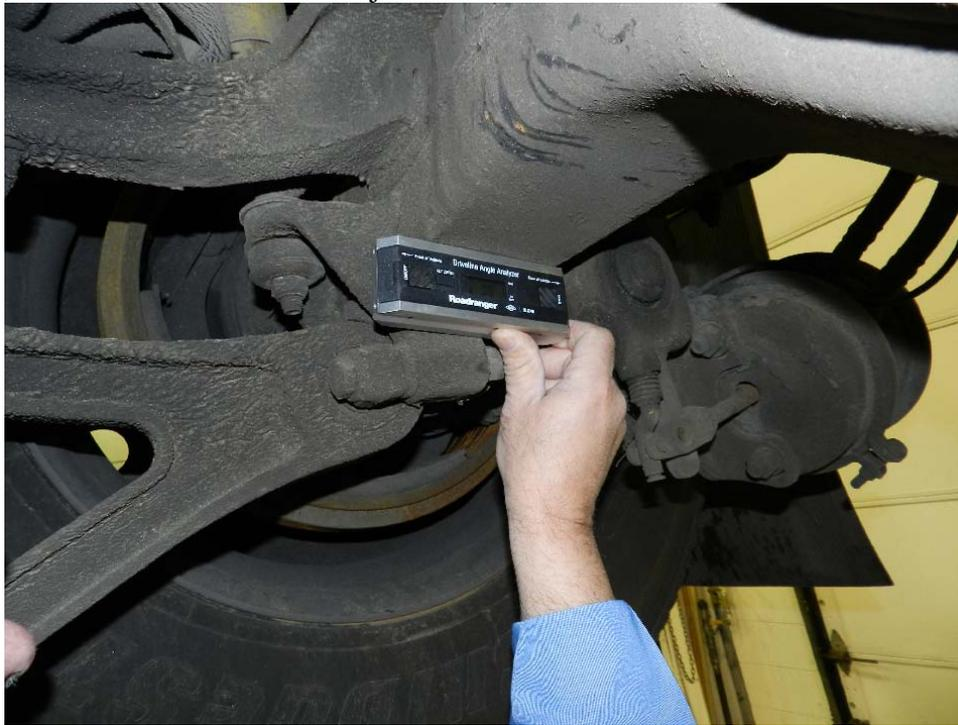
After all of the component angles are measured with the digital protractor, they may be entered in the DAA program. First enter all of the required information on the Information page. Be sure to enter the driveline and axle models. This will allow you to use the corrective action utility.
