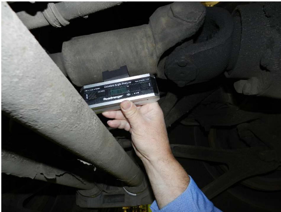
Finally, measure the rear drive axle just as the front drive was done.
