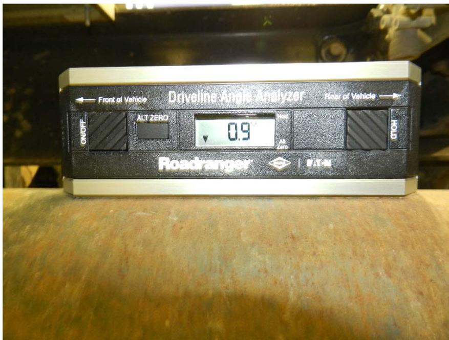
Next, measure the front axle on the arm of the axle near the spring mounts. This measurement may be made at the bottom or top of the arm.
