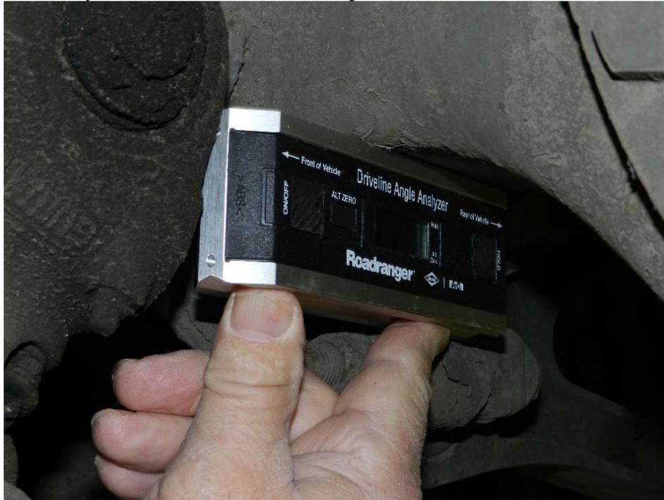
Next measure the interaxle drive shaft. A v-block is available to assure that the measurement can be made without weld interference.
