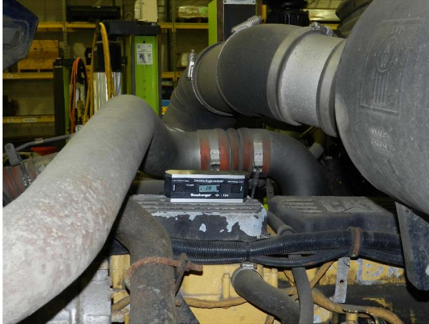
Next, measure the angles of the various main drive shafts. Make as many measurements as there are drive shaft segments. These measurements may be made at the top or the bottom of the shaft. Heed the direction of the arrows “Front of Vehicle” and “Rear of Vehicle”. Note also the arrow pointing down at the left of the LED. This reading is a positive 0.9 degree angle with a downward slope toward the rear of the vehicle. (See Rules)
